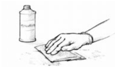
Figure 6 Clean the surface. Use a solvent, if necessary, to remove all contaminants.
