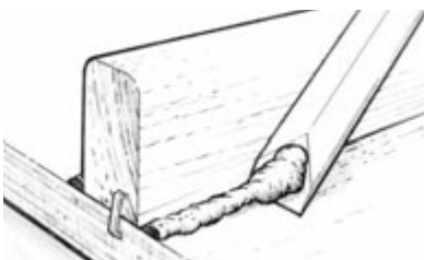
Figure 12 Remove or shape excess epoxy that squeezes out of the joint.
