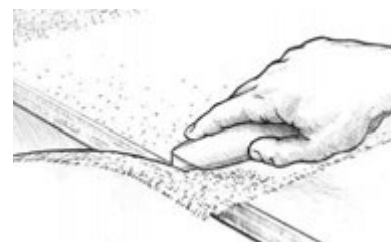
Figure 26 Trim excess cloth after the epoxy gels.
