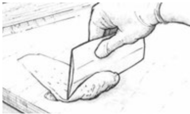
Figure 22 Apply fairing compound to fill all voids and smooth to shape.
