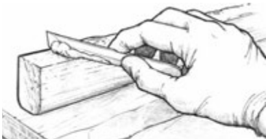
Figure 10 Apply thickened epoxy to one of the bonding surfaces.
