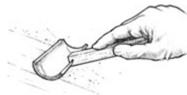
Figure 31 Tip off the coating by dragging a foam roller brush lightly over the fresh epoxy.
